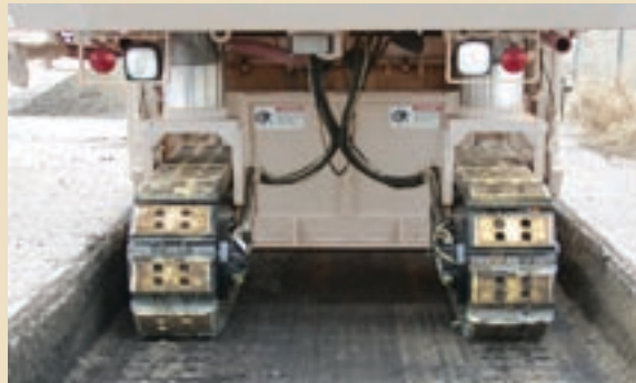
PR600C's power makes 14 in (355 mm) deep plunge cuts easy.
