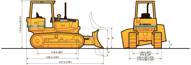
\* Overall height with Cab ROPS - 2.76 m (108.5") Vertical dimensions include 53.6 mm (2.11") grouser height
