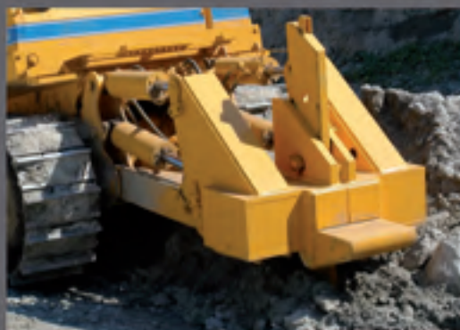
Single-shank and multi-shank rippers are equipped with hydraulic pitch.
