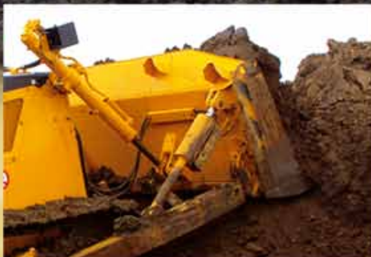
Semi-U blades of 7.45 cu.yd (5.7 cu.m) for STD & LT track frame and 7.8 cu.yd (5.95 cu.m) for WT version, combine penetration ability of straight blade with increased capacity provided by short wings. The blades can be equipped with tilt or tilt/pitch option.
