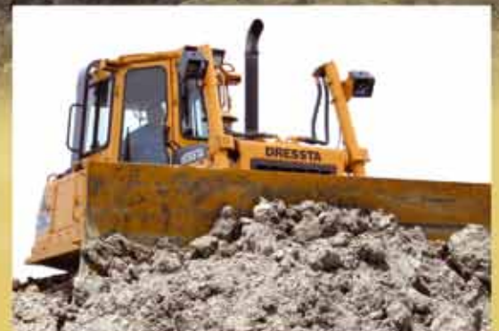
Angle blade of 5 cu.yd (3.8 cu.m) used with STD & LT track frame, is ideal for side-casting, backfilling, cutting ditches or setting a final grade by reducing amount of maneuvering required to do these jobs. 2-cylinder blade tilt is offered as an option.
