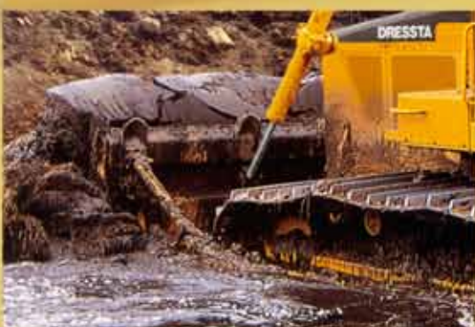
Straight blade of 4.7 cu.yd (3.6 cu.m) used with 85 in (2.16 m) gauge and 37 in (940 mm) track shoes (LGP) is designed for soft, swampy areas. This blade may be equipped with hydraulic tilt cylinder to perform efficiently landscaping operations.
