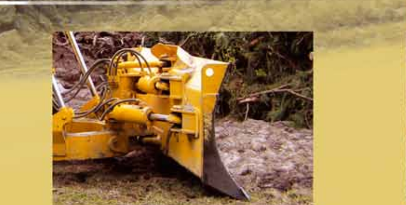
6-way hydraulic angle blade of 5 cu.yd (3.8 cu.m) used with 80 in (2.03 m) gauge wide track (WT) and max. shoe width of 22 in (560 mm) is applicable for versatile operations such as finish grading, spreading material and light land clearing.
