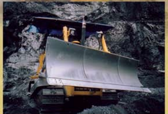
Angle blade of 3.8 cu.m (5 cu.yd) used with STD&LT track frame, is ideal for side-casting, backfilling, cutting ditches or setting a final grade by reducing amount of maneuvering required to do these jobs. 2-cylinder blade tilt is offered as an option.
