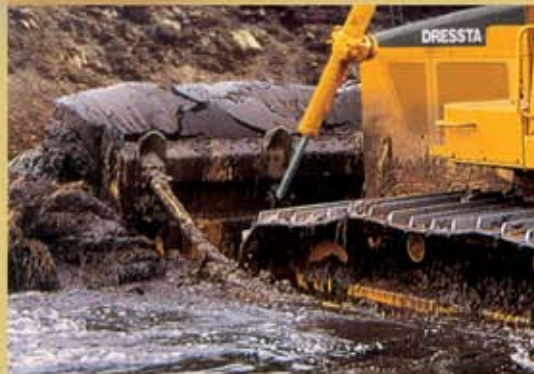
Straight blade of 3.6 cu.m (4.7 cu.yd) used with 2.16 m (85 in) gauge and 940 mm (37 in) track shoes (LGP) is designed for soft, swampy areas. This blade may be equipped with hydraulic tilt cylinder to perform efficiently landscaping operations.
