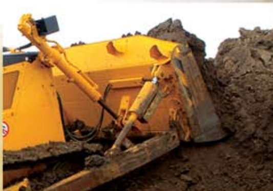
Semi-U blades of 5.7 cu.m (7.45 cu.yd) for STD&LT track frame and 5.95 cu.m (7.8 cu.yd) for WT version, combine penetration ability of straight blade with increased capacity provided by short wings. The blades can be equipped with tilt or tilt/pitch option.
