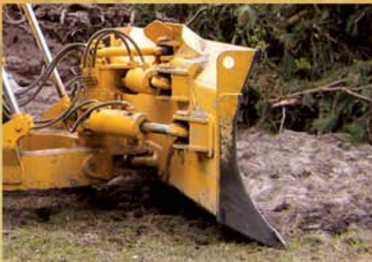
6-way hydraulic angle blade of 3.8 cu.m (5 cu.yd) used with 2.03 m (80 in) gauge wide track (WT) and max. shoe width of 560 mm (22 in) is applicable for versatile operations such as finish grading, spreading material and light land clearing.
