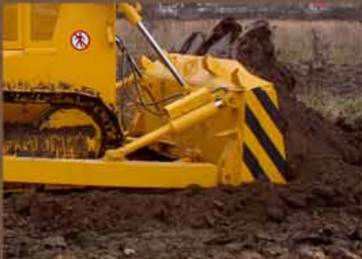
Semi-U blade of 5.6 yd 3 (4.28 m 3 ) (STD)
