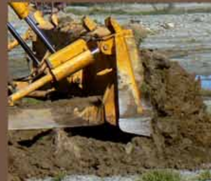
Straight blade of 4.0 yd 3 (3.05 m 3 ) (STD)
