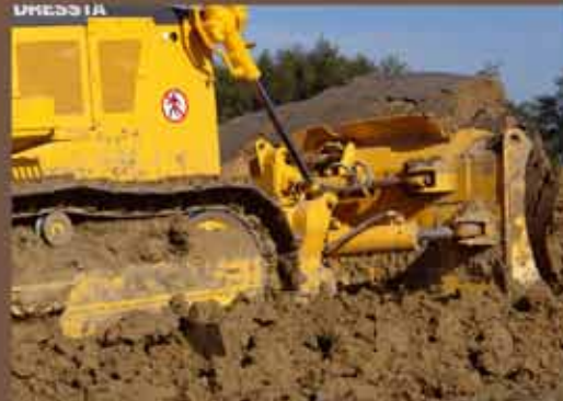
6-way hydraulic angle blade of 4.2 yd 3 (3.2 m 3 ) (STD & LT) and 5.0 yd 3 (3.8 m 3 ) (LGP)
