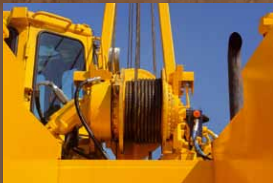
Two independently controlled hydraulic winches drive the boom and hook systems.
